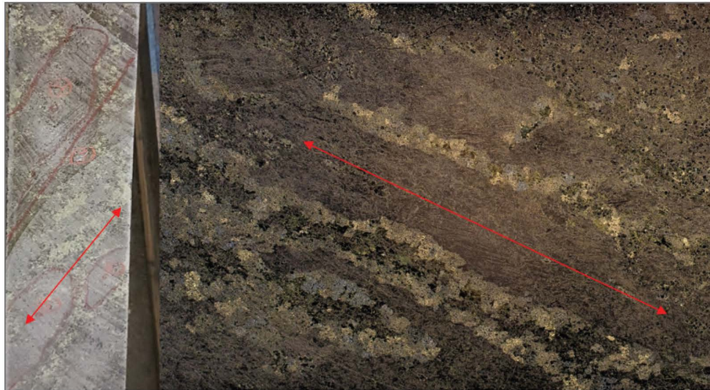
Hole EL-17-14 @ 136.1m Stretched loop textured pyrrhotite-pentlandite-chalcopyrite massive sulphide. Lineation indicates flow directions (red line)
