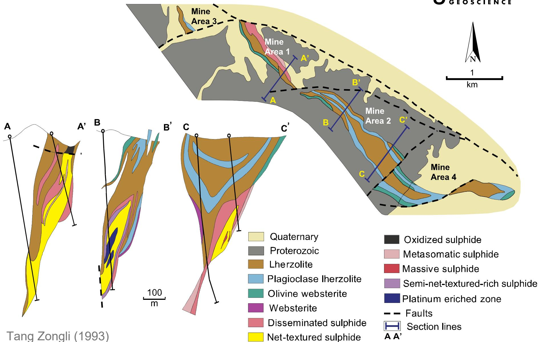
Mine area #2 – no trace of sulfide or country rock xenoliths inside the intrusion at surface
