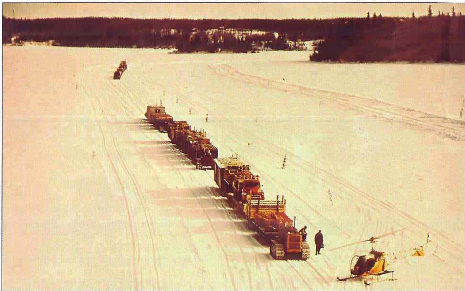
SNOWBALL EXPRESS A system of tractor trains worked night and day during the winter of 1956-57 to move more than 30,000 tons of material and equipment from the rail head at Thicket Portage to the mine site. The 70-mile round trip took 14 hours.
